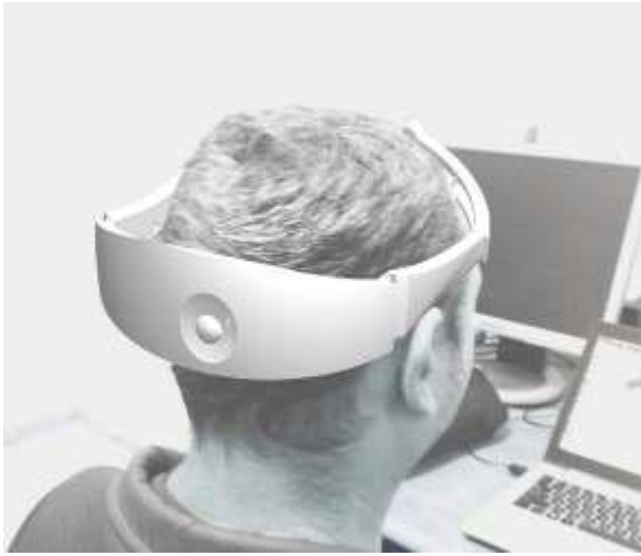
Fig. 1 - Backview illustrative embodiment of a transcranial 580 electrotherapy brain stimulator device
